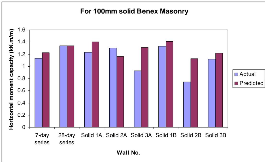
Figure 36. Comparison of Benex horizontal beam results with predicted capacities for solid block masonry
