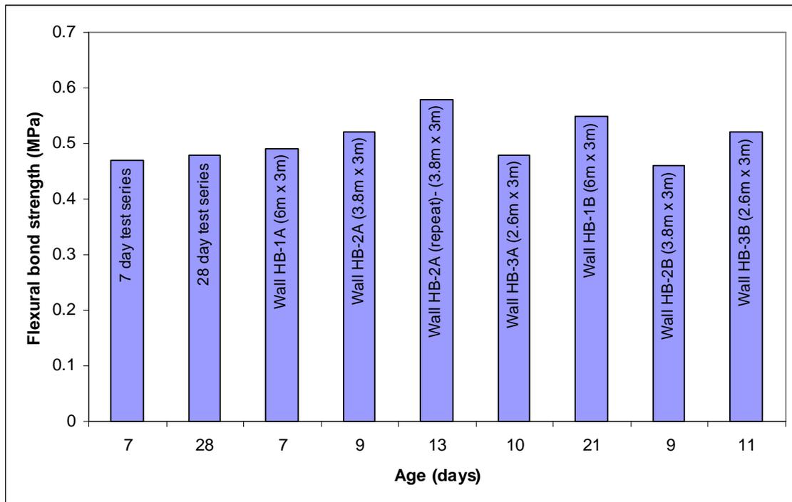
Figure 26. Average flexural bond strength at different ages of 200mm thick hollow Benex masonry
