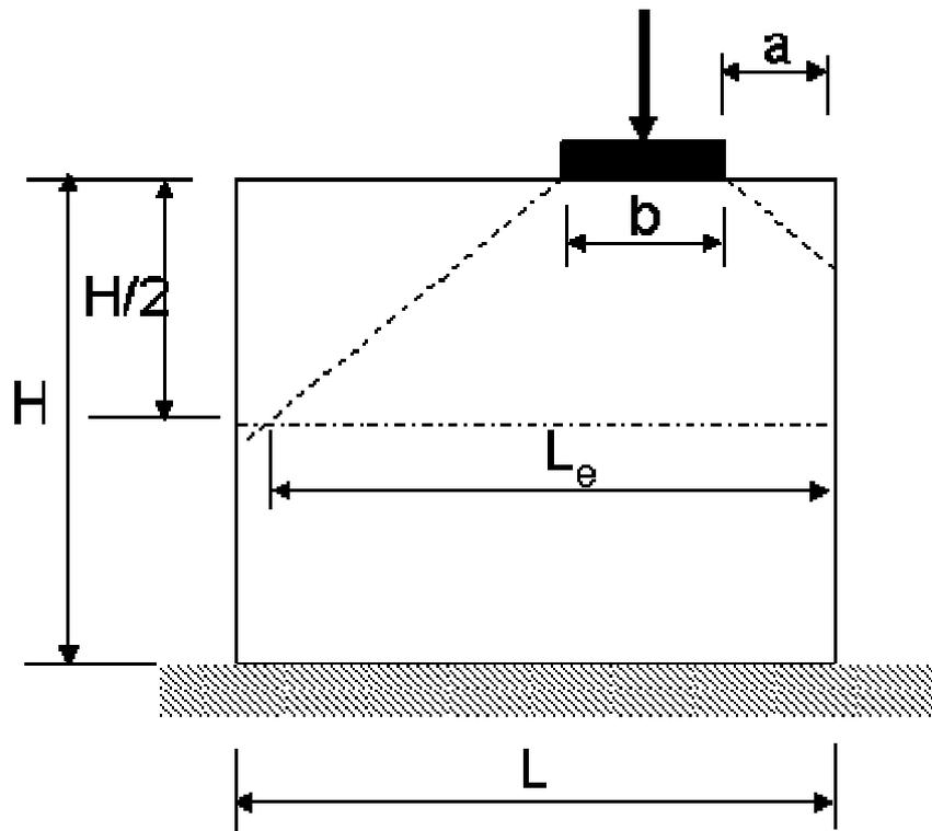
Figure 16. Load dispersion under concentrated load
