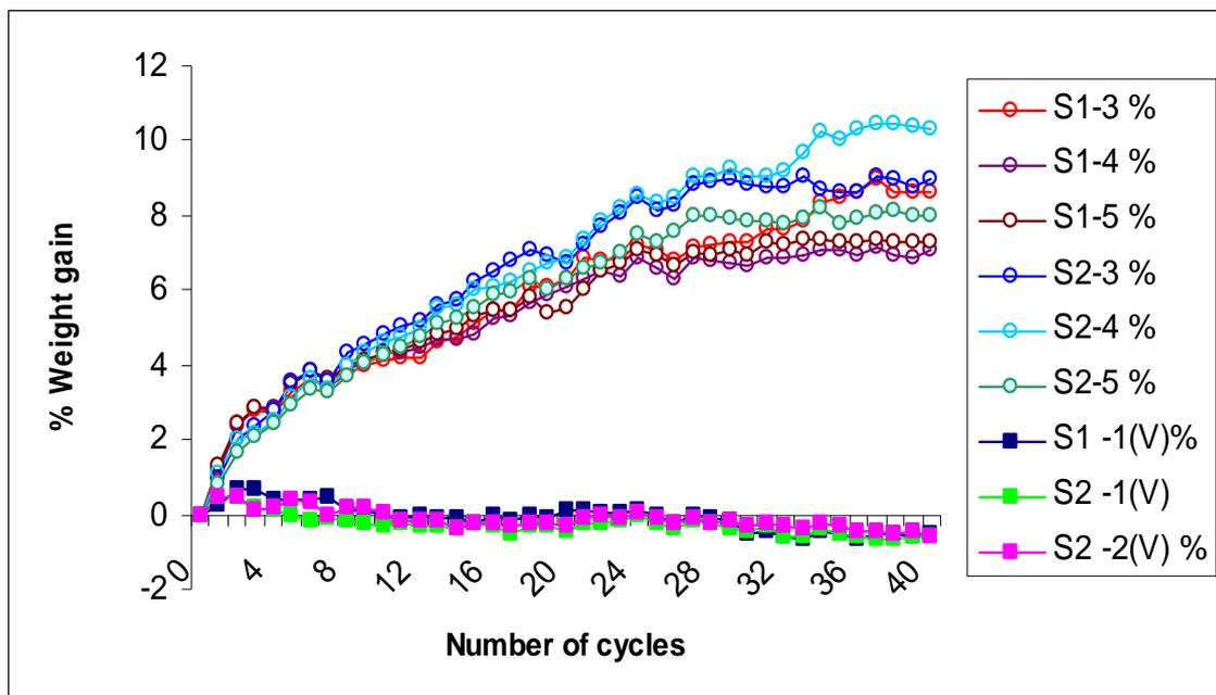
**Figure 10.** Percentage weight change of specimens taken from solid blocks (Vaseline treated samples contain “V” in the name)
