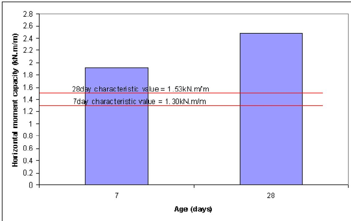
Figure 32. 7-day & 28-day horizontal moment capacities of 200mm thick hollow Benex masonry
