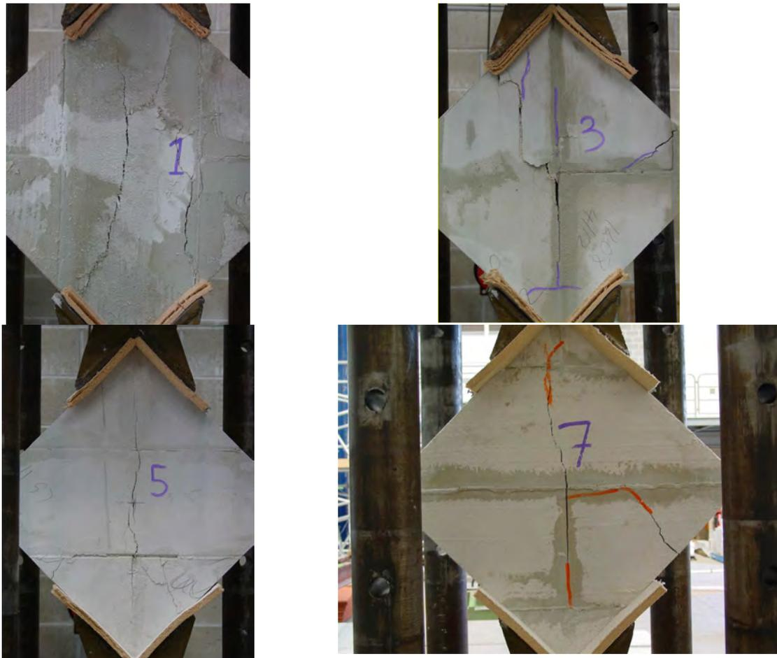
**Figure 53.** Typical failure modes of 100mm thick solid Benex masonry under diagonal load
