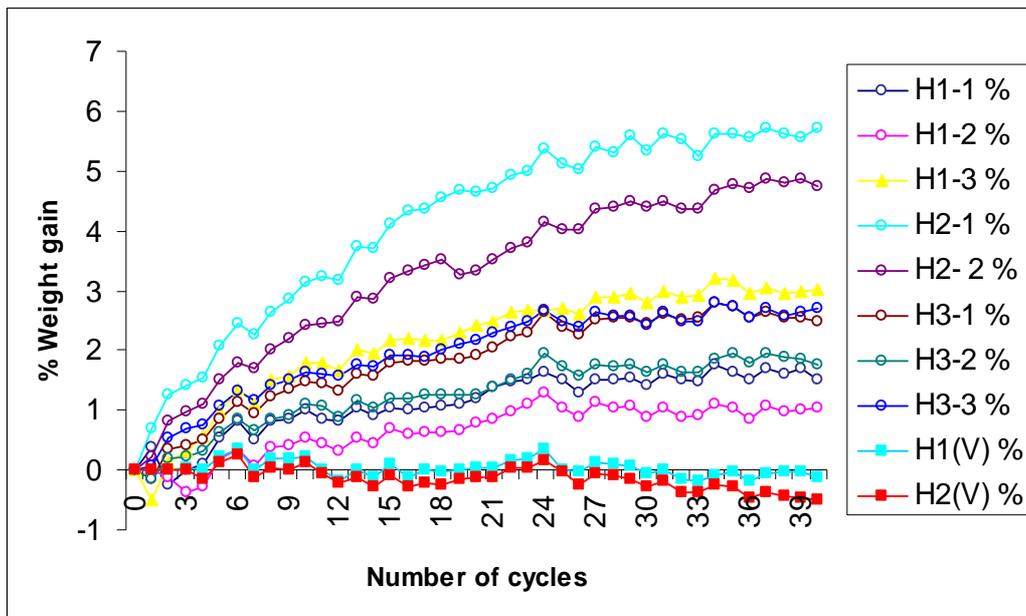
**Figure 11.** Percentage weight change of specimens taken from hollow blocks (Vaseline treated samples contain “V” in the name)
