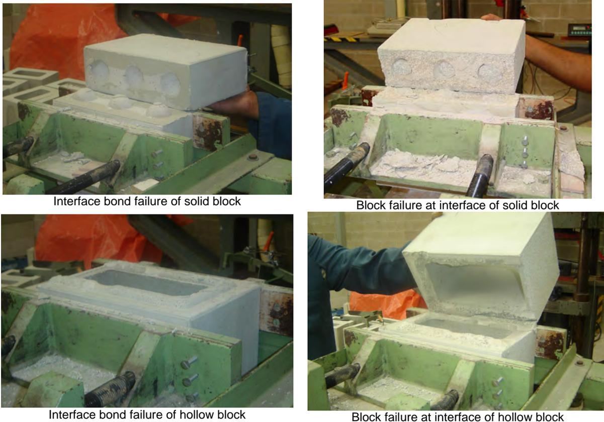
**Figure 27.** Modes of flexural bond failures
