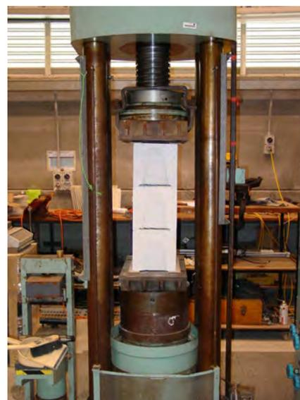
(b) 200mm thick hollow block masonry
