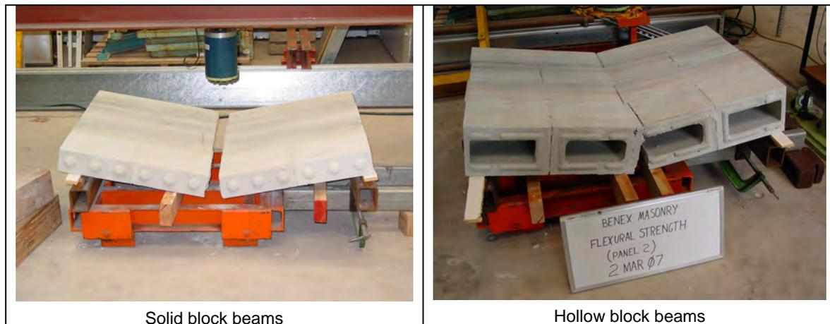
**Figure 35.** Typical failures of specimen subjected to horizontal bending
