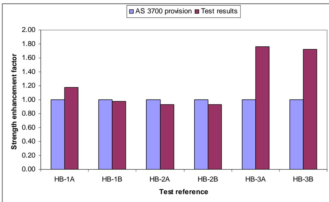
**Figure 21.** Strength enhancement factor under concentrated loads for hollow blocks
