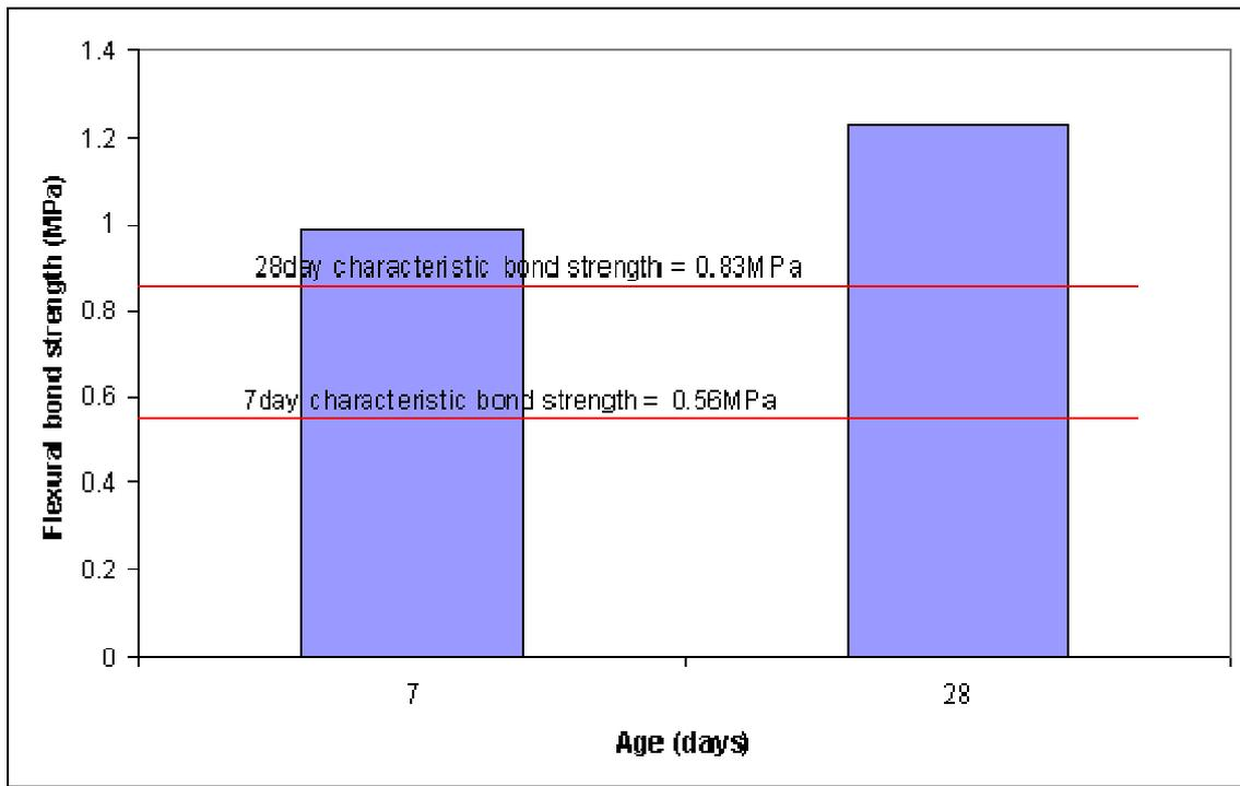
Figure 23. 7-day & 28-day flexural bond strength of 100mm thick solid Benex masonry
