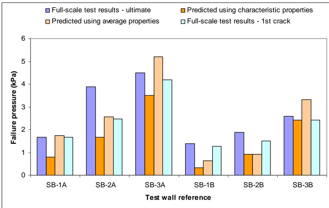
Figure 46. Predicted failure pressures for 100mm solid block masonry
