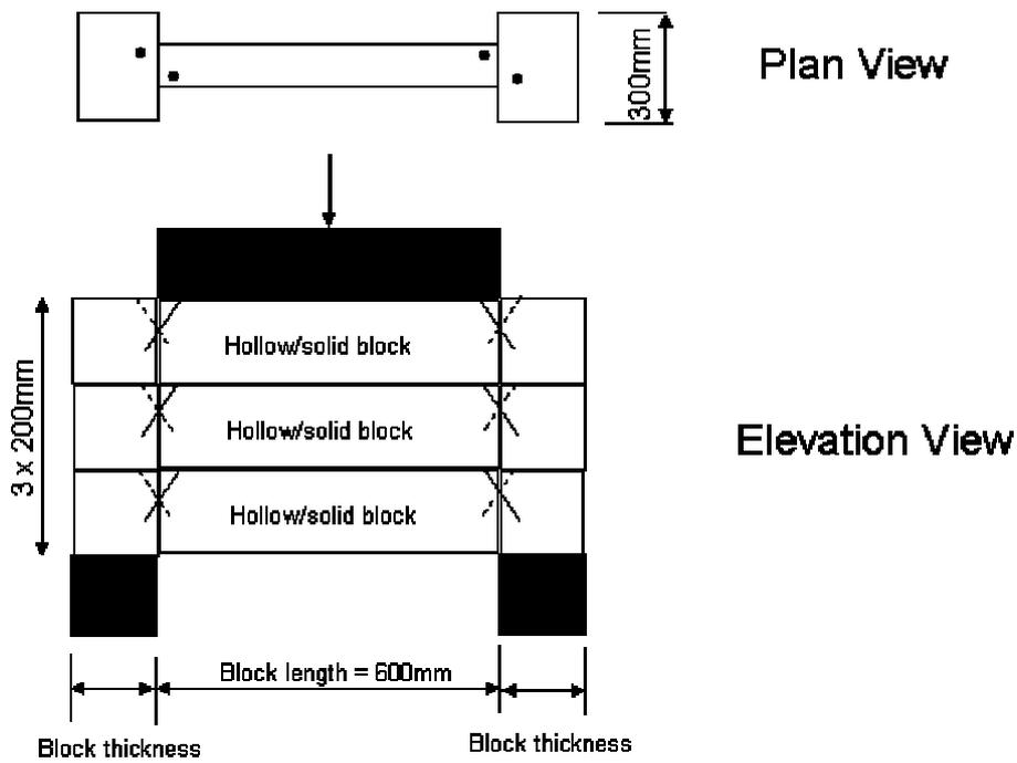
Figure 62. Schematic diagram of the test set up
