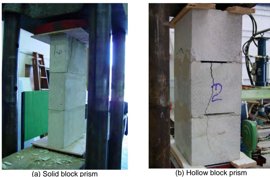
**Figure 15.** Typical failure of a prism under compression
