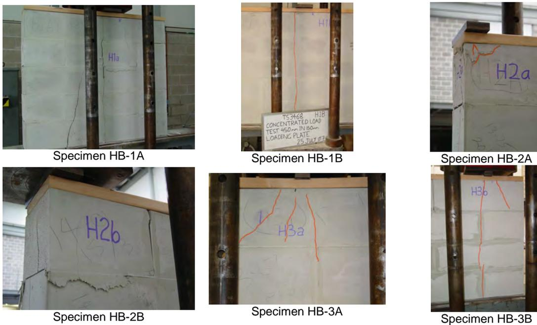
Figure 19. Failure modes – Hollow block wall specimens
