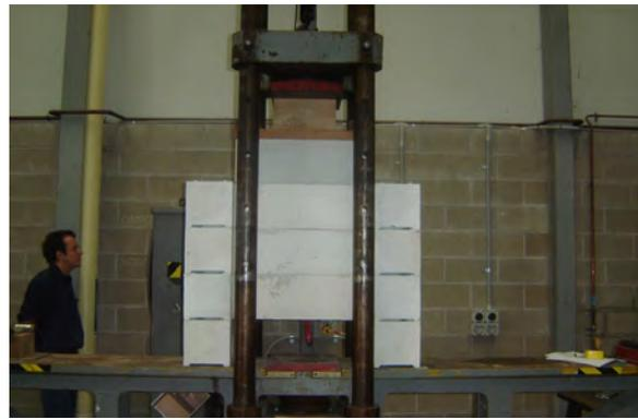
Hollow block and hollow block interface
