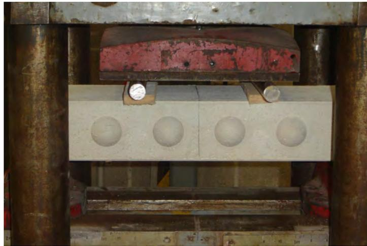
**Figure 28.** Test set up for modulus of rupture of Benex solid block
