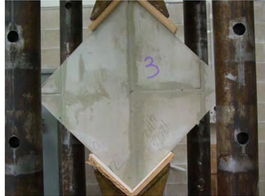
Loading parallel to bed joint along a joint with joint intersection at the centre of the 400mm square panel
