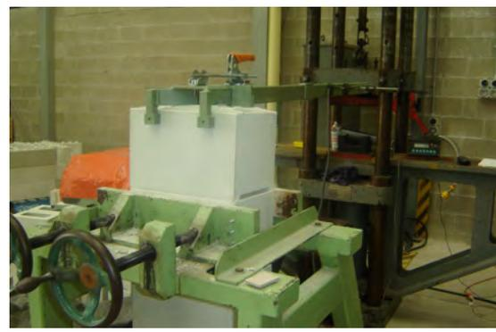
200mm hollow block under test
