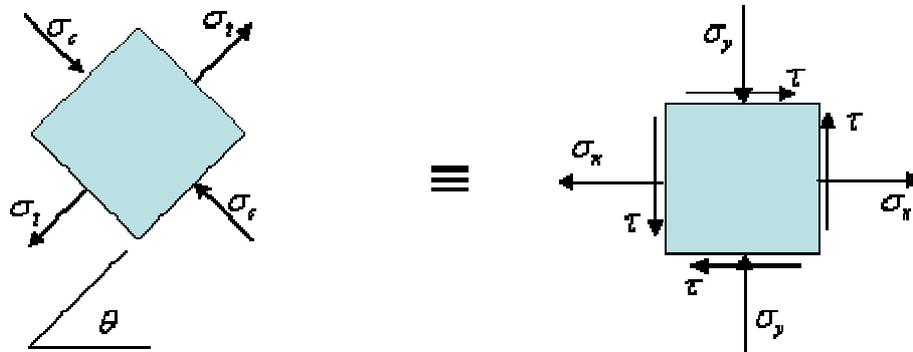
**Figure 57.** Stresses within an element in the wall subjected to racking shear
