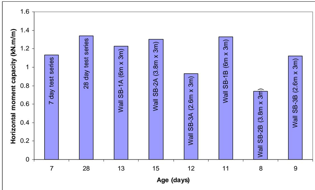
Figure 33. Average horizontal moment capacity at different ages of 100mm thick solid Benex masonry
