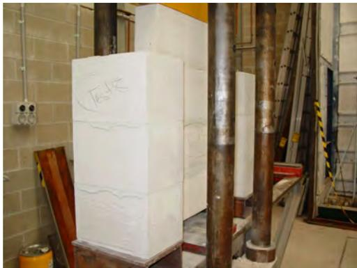
hollow block and solid block wall interface
