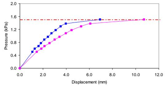
Figure 40 (e). Crack pattern and deflection at centre for solid block wall (3.8m x 3m) supported on 3 sides with top side free
