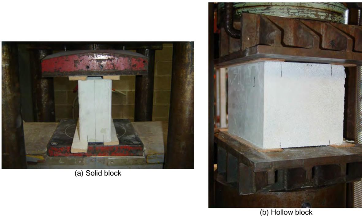
**Figure 12.** Test set up for compression on hollow & solid blocks
