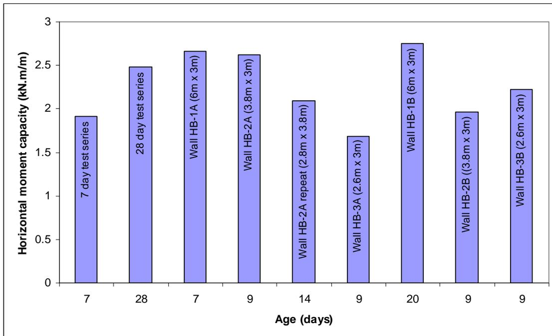
Figure 34. Average horizontal moment capacity at different ages of 200mm thick hollow Benex masonry
