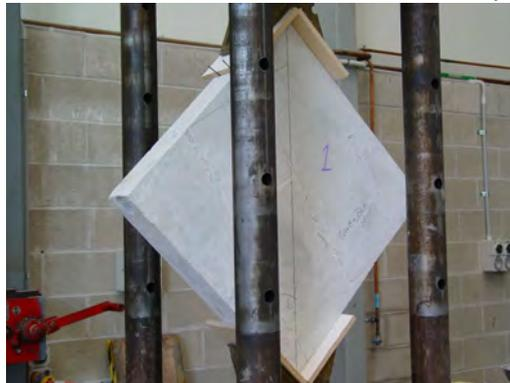
Loading approximately at  $30^\circ$  to bed joint with a joint intersection at the centre of the 600mm square panel
