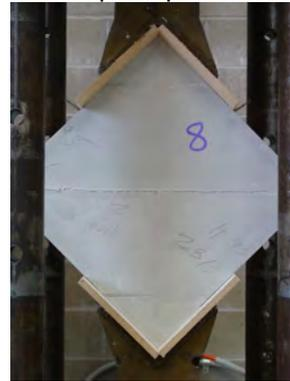
Loading perpendicular to bed joint with a joint intersection at the centre of the 400mm square panel
