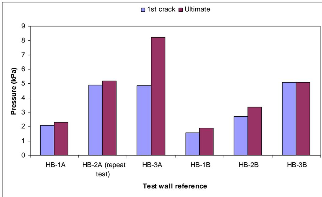
Figure 43. Failure pressures of test walls built with 200mm hollow blocks
