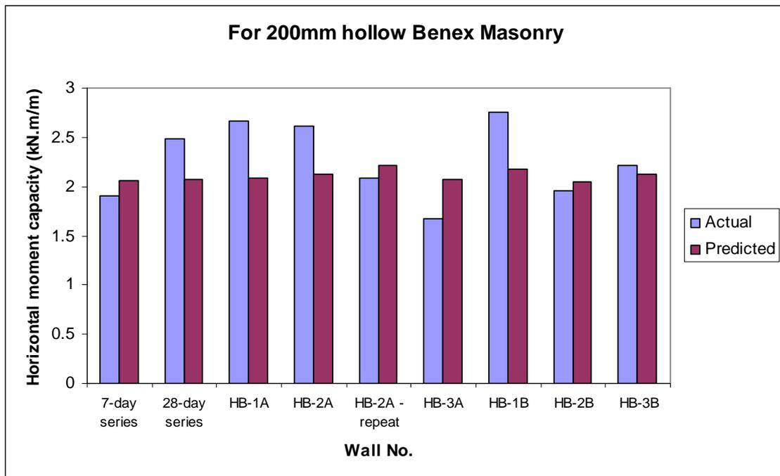
Figure 37. Comparison of Benex horizontal beam results with predicted capacities for hollow block masonry
