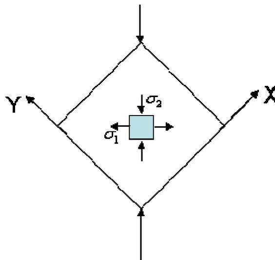
**Figure 58.** Stresses within an element in a wall subjected to a diagonal load
