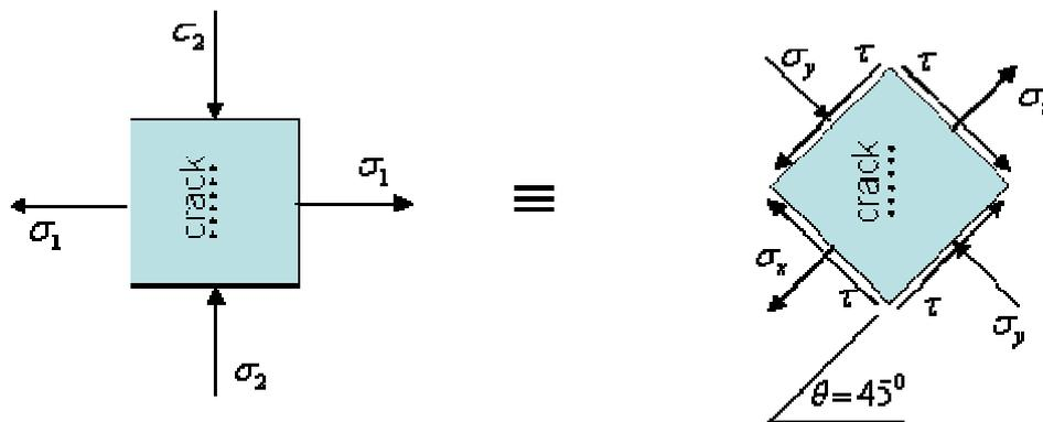
Figure 59. Principal stresses converted to normal stresses
