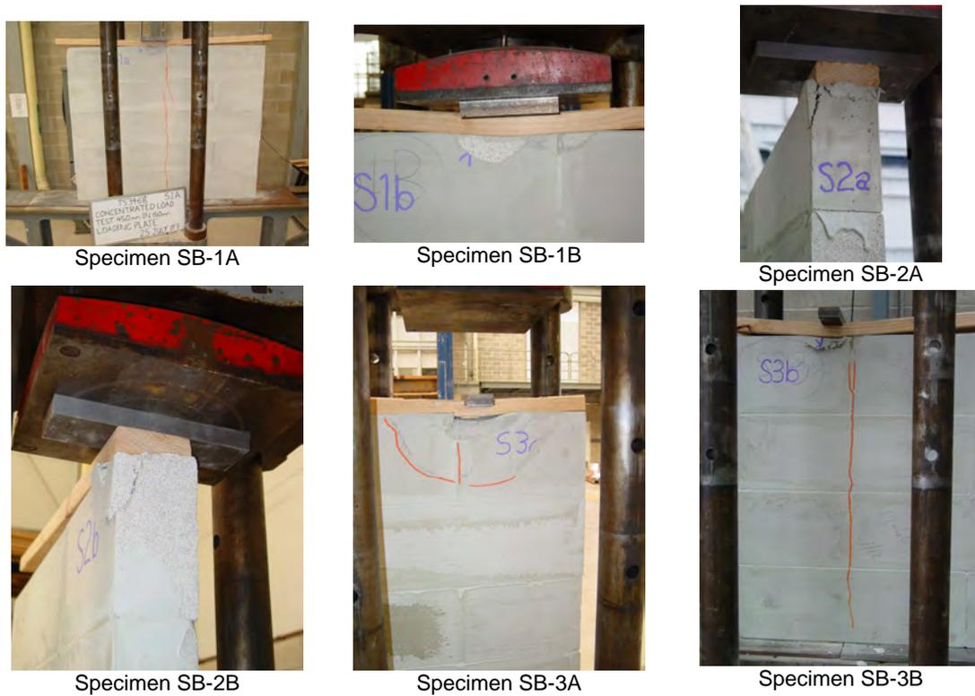
Figure 18. Failure modes – Solid block wall specimens
