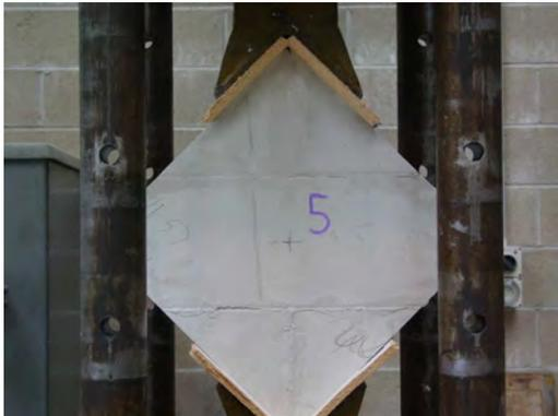
Loading perpendicular to bed joint with a block at the centre of the 400mm square panel
