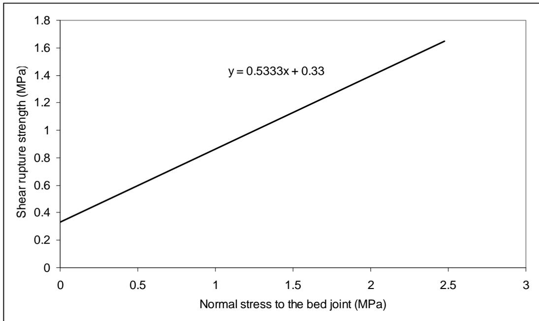
**Figure 61.** Relationship between shear rupture and normal stress for 200mm thick hollow Benex masonry
