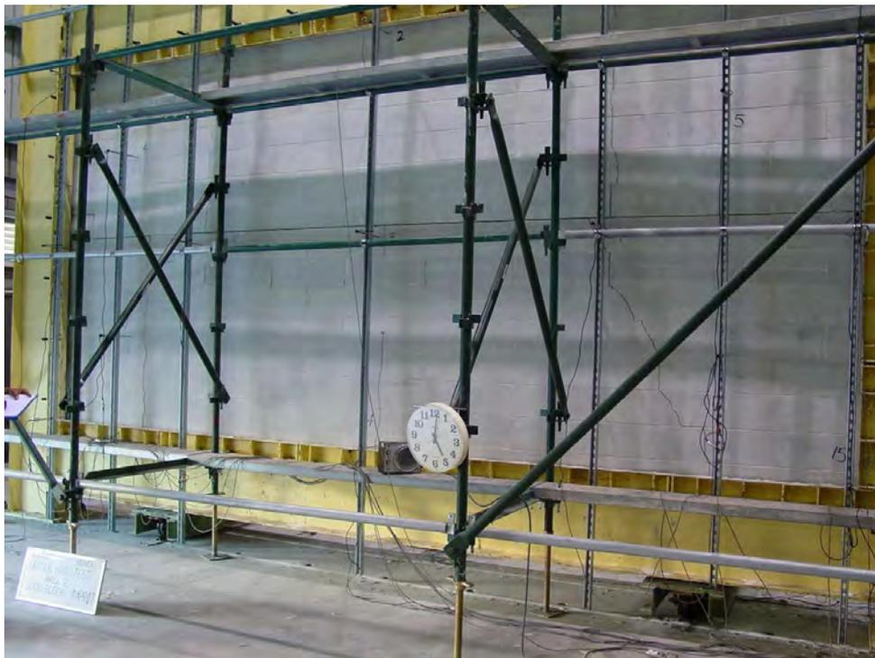
**Figure 39.** Lateral load test set up
