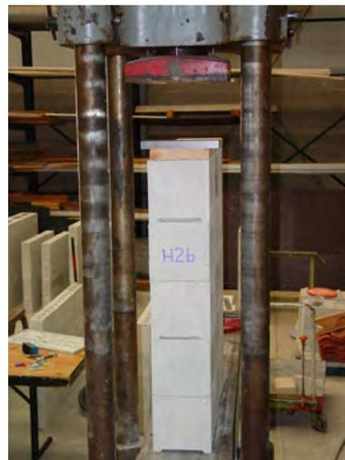
(b) Hollow block wall – set up for edge loading
