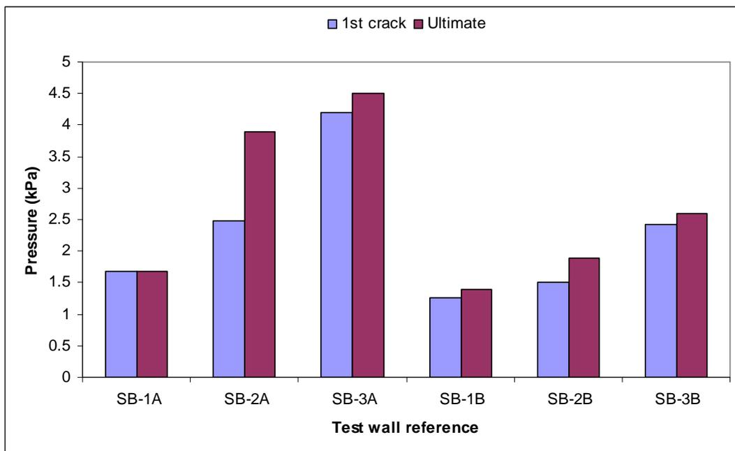
Figure 42. Failure pressures of test walls built with 100mm solid blocks
