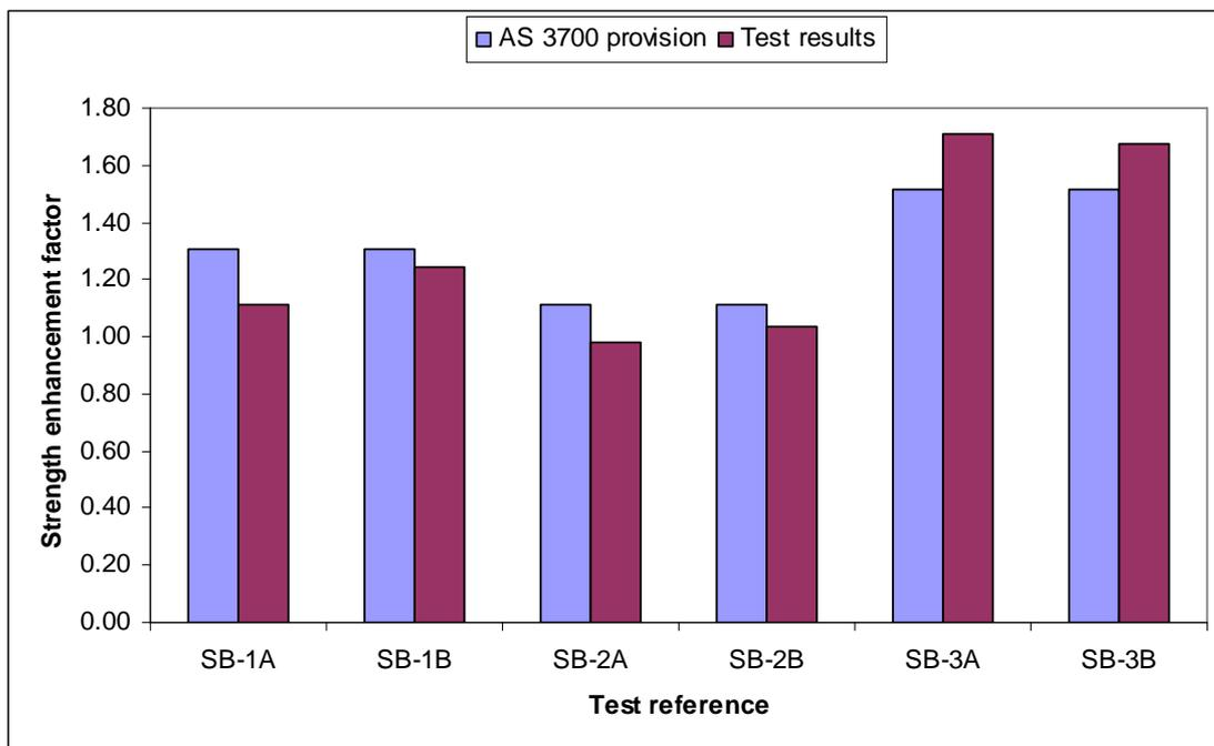
**Figure 20.** Strength enhancement factor under concentrated loads for solid blocks
