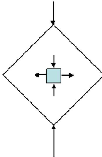
Figure 55. Schematic diagram showing principal stresses at the centre of panel under diagonal loading
