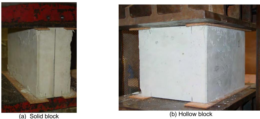
**Figure 13.** Typical failures of blocks under compression
