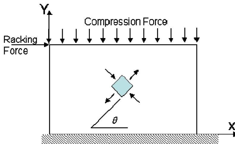
Figure 56. Schematic diagram showing principal stresses within a wall subjected to racking shear
