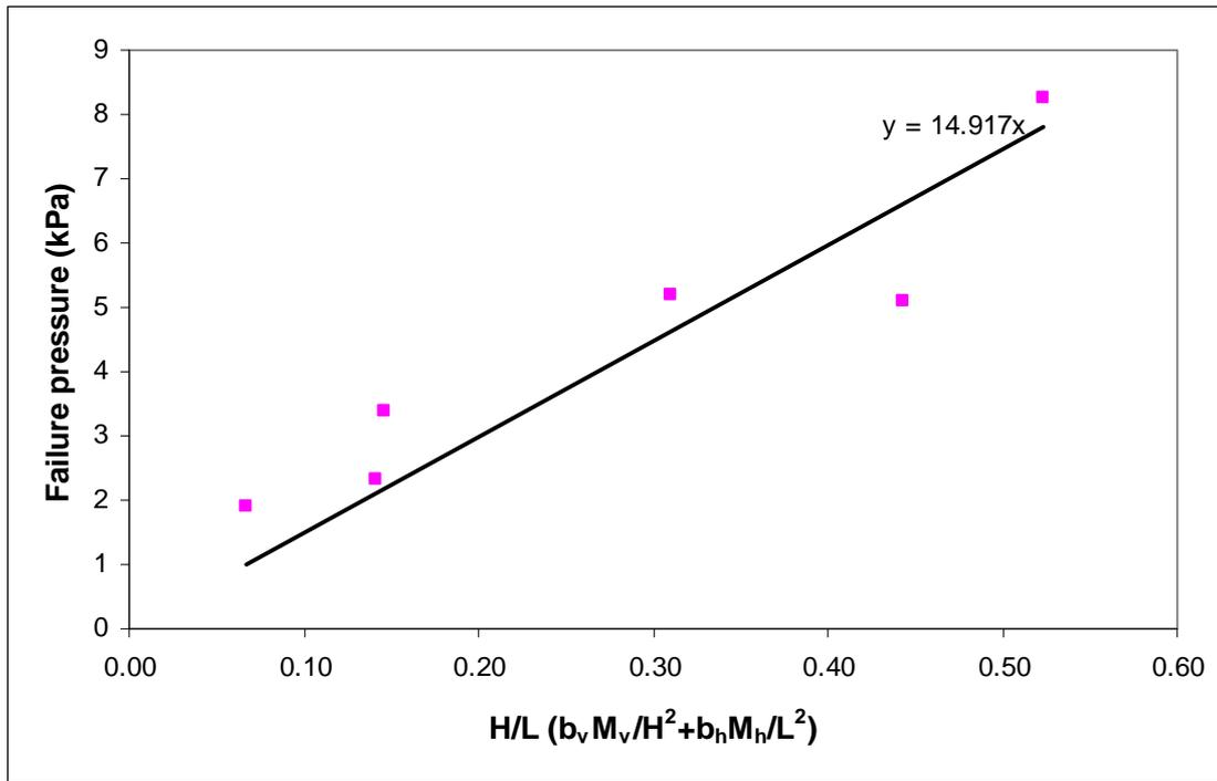
Figure 45. Assessment of “k” for 200mm hollow block masonry
