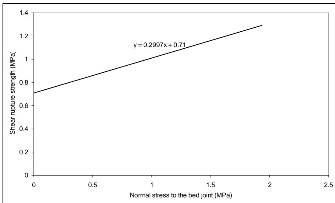
**Figure 60.** Relationship between shear rupture and normal stress for 100mm thick solid Benex masonry
