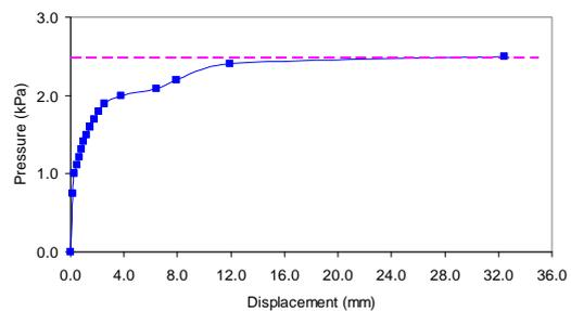
Figure 40 (b). Crack pattern and deflection at centre for solid block wall (3.8m x 3m) supported on all 4 sides
