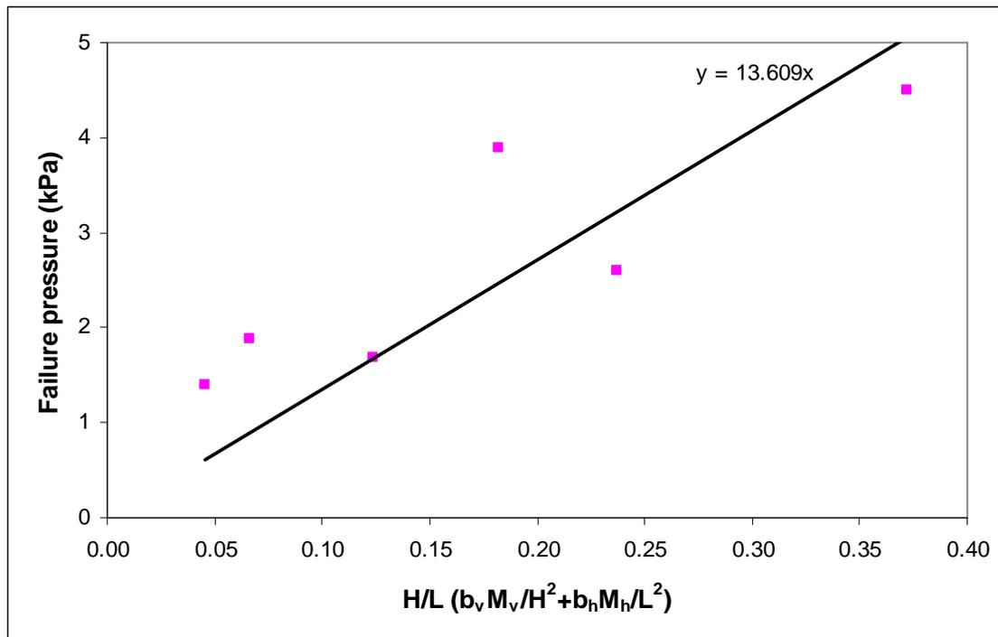
**Figure 44.** Assessment of “k” for 100mm solid block masonry
