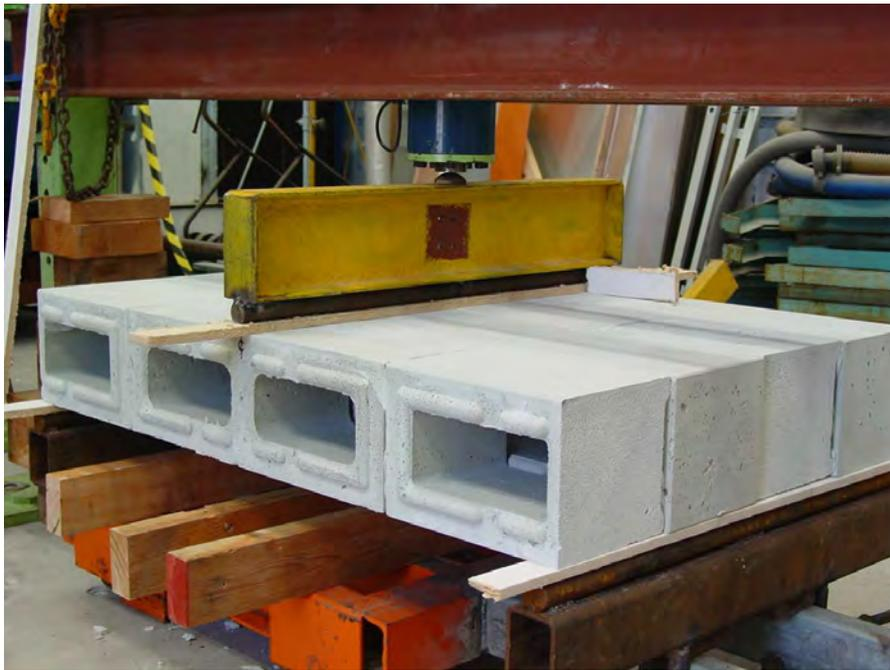
**Figure 30.** Test set up for horizontal beam test
