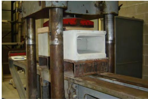
**Figure 50.** Out-of-plane shear test set up
