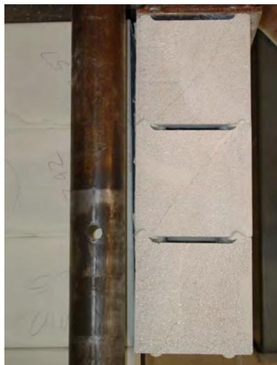
**Figure 67.** A typical interface shear failure at the butted face
