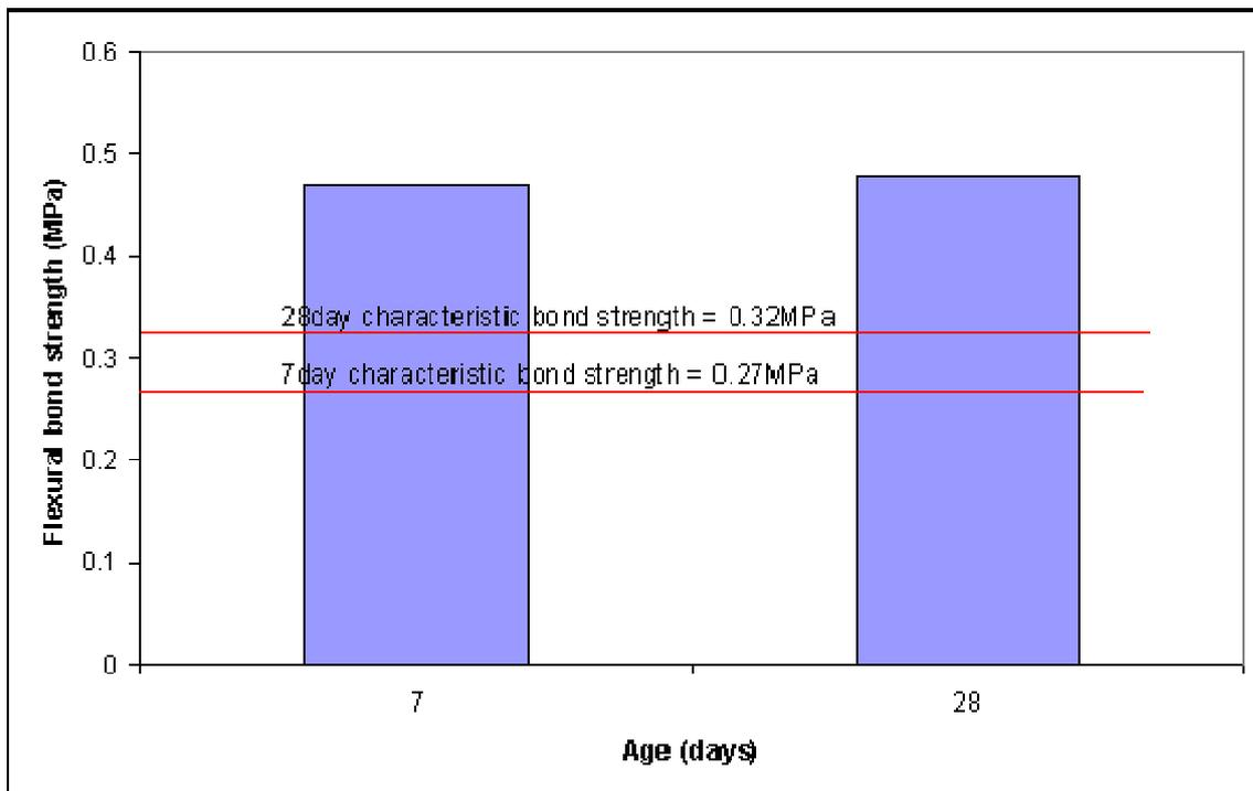
Figure 24. 7-day & 28-day flexural bond strength of 200mm thick hollow Benex masonry
