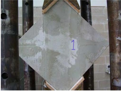
Loading parallel to bed joint with a block at the centre of the 400mm square panel
