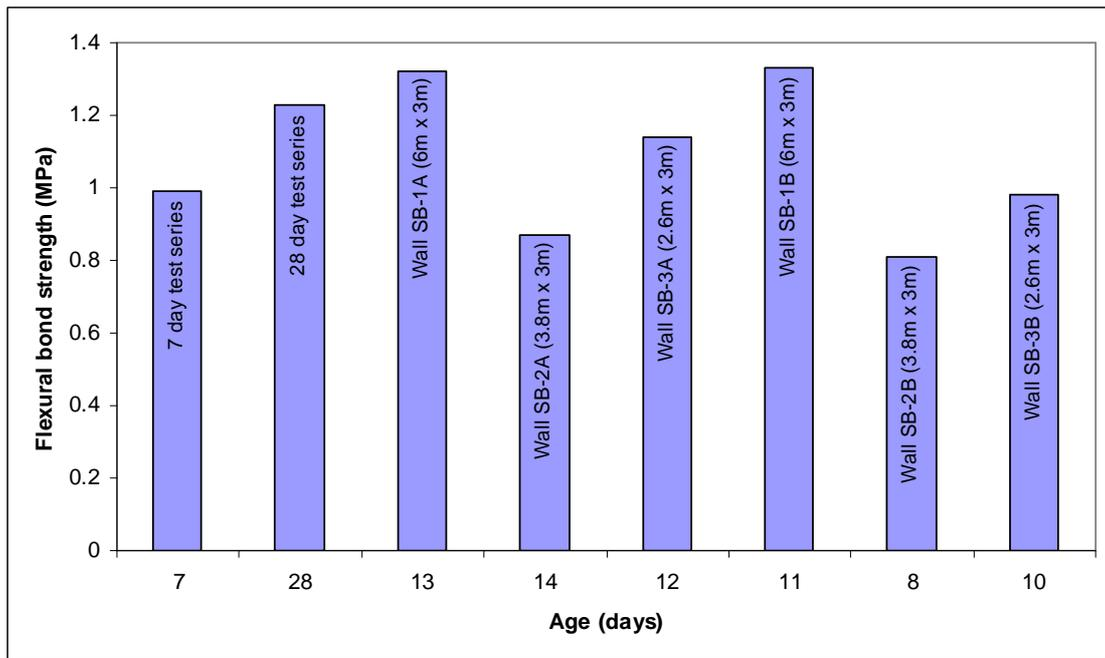
Figure 25. Average flexural bond strength at different ages of 100mm thick solid Benex masonry
