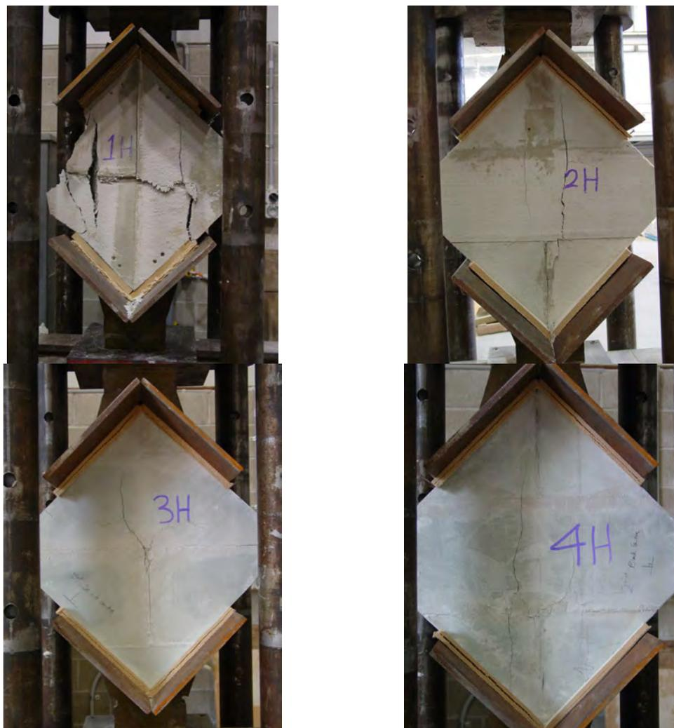
**Figure 54.** Typical failure modes of 200mm thick hollow Benex masonry under diagonal load
