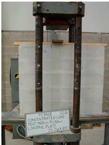
(a) Solid block wall – set up for mid length loading
