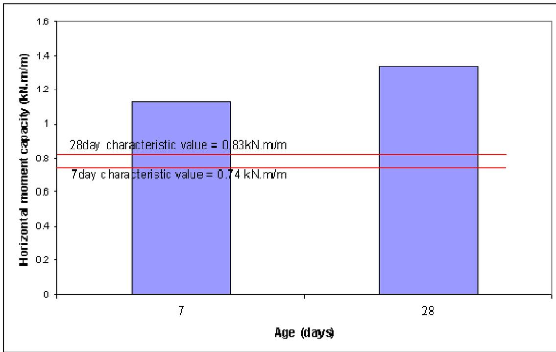
Figure 31. 7-day & 28-day horizontal moment capacities of 100mm thick solid Benex masonry
