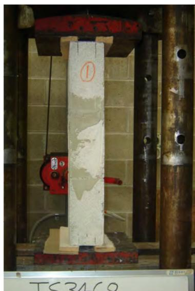
(a) 100mm thick solid block masonry
