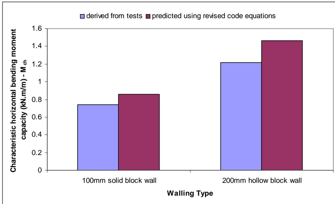
Figure 38. Comparison of Benex 7-day horizontal beam results with recommended formulae
