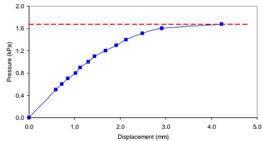
Figure 40 (a). Crack pattern and deflection at centre for solid block wall (6m x 3m) supported on all 4 sides
