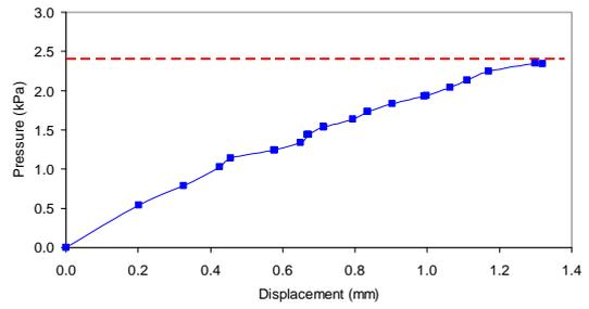
Figure 41 (b). Crack pattern and deflection at centre for hollow block wall (3.8m x 3m) supported on all 4 sides
