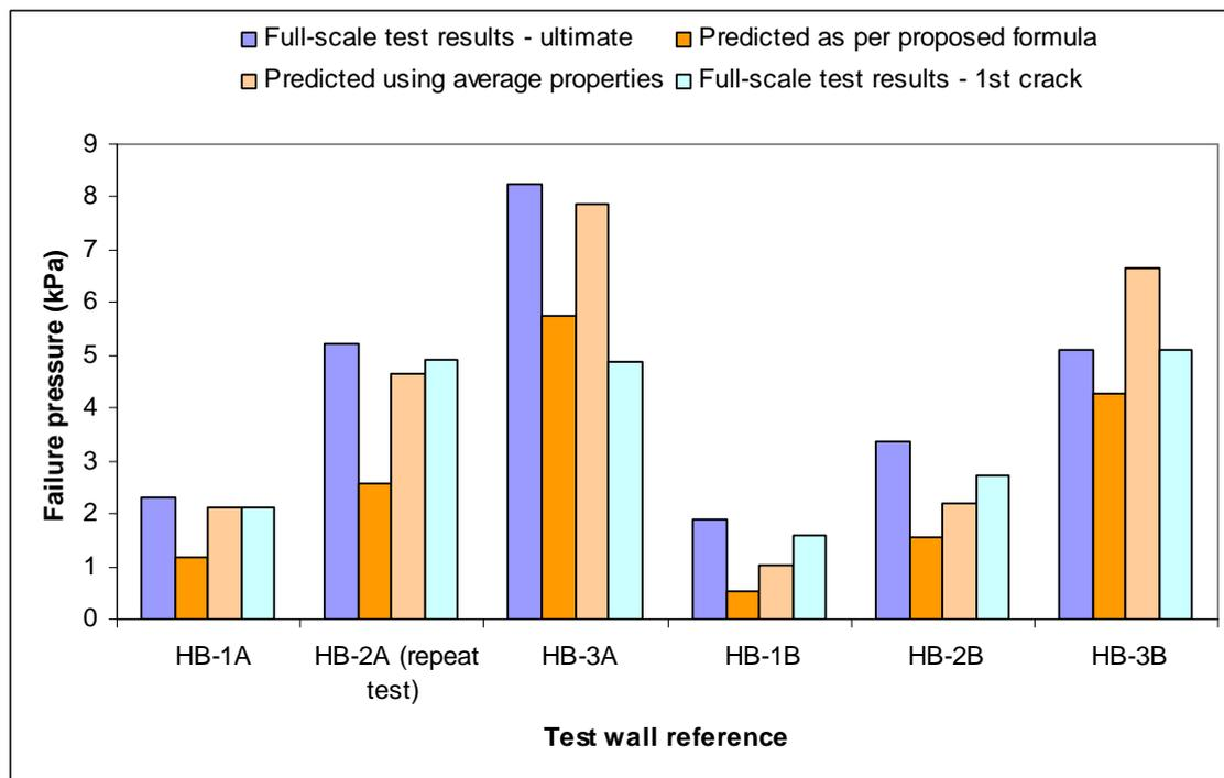
Figure 47. Predicted failure pressures for 200mm hollow block masonry
